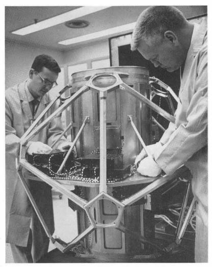
ASSEMBLING logics systems in the test detection satellite frame are W. B. Goldrick (7432-2) and F. E. Thompson, 7432-2 supervisor, right. Holes at the triangular points of the frame will contain LASL-designed X-ray detectors. Solar cells will power the satellite instrumentation.
